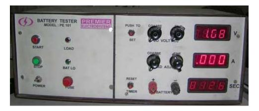
Premier's Battery Tester are suitable for testing different Batteries for monitoring its Load Characteristics.
